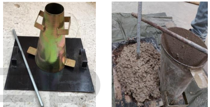
Figure 2: The performed slump test.
