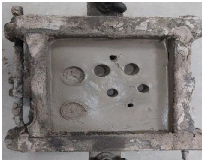
Figure 11: mould of Setting Time Test.
